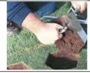
Each unit includes a trowel allowing for uniform plug depth
