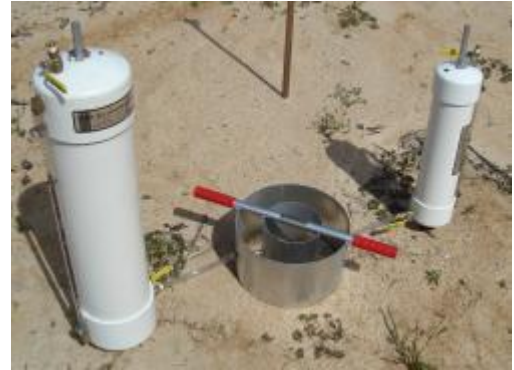
Photo showing IN8P-W Turf-Tec Heavy Duty Tall Infiltration Rings - 6 and 12 inch diameter by 7 inches tall with ports for optional Mariotte Tubes - Ports are located three inches from bottom of rings allowing three inch insertion into the soil and five inches of water on top of soil.
