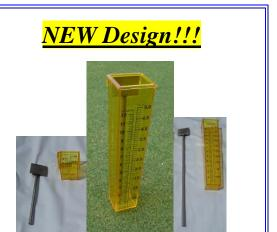
Precipitation and Uniformity Gauges have a stainless steel support spike and are calibrated in 10th of an inch and millimeters. Smaller gauges are positioned next to sprinkler heads to catch the second or third lower stream from the nozzles.
