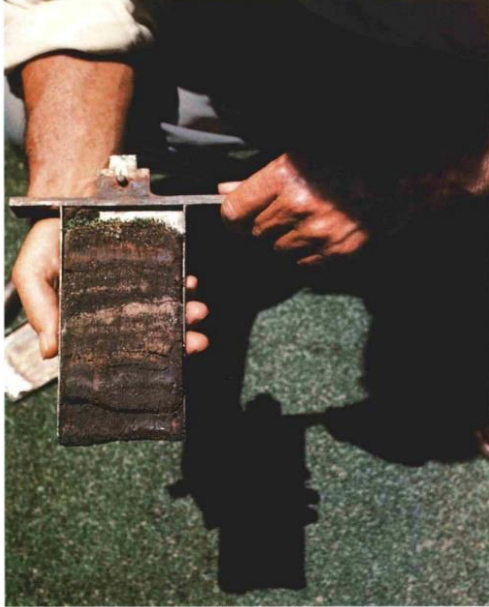
Several layers, created by topdressing with different materials, represent different management programs over the years.
