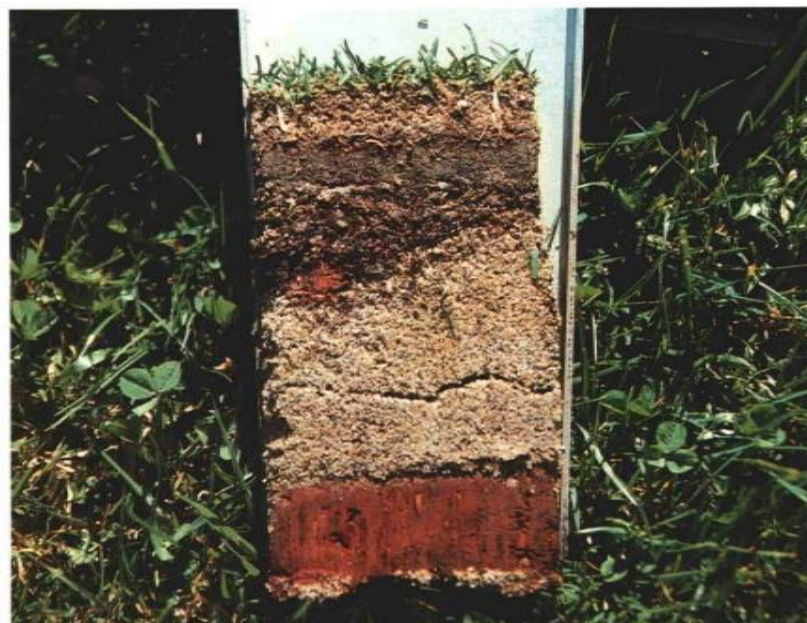
This profile indicates how poorly the soil was mixed during construction. Concentration of any one of the soil components creates problems in water movement and root development in the profile.
