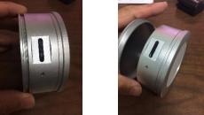
2. Install rechargeable battery as shown below. Be sure battery polarity is correct.
