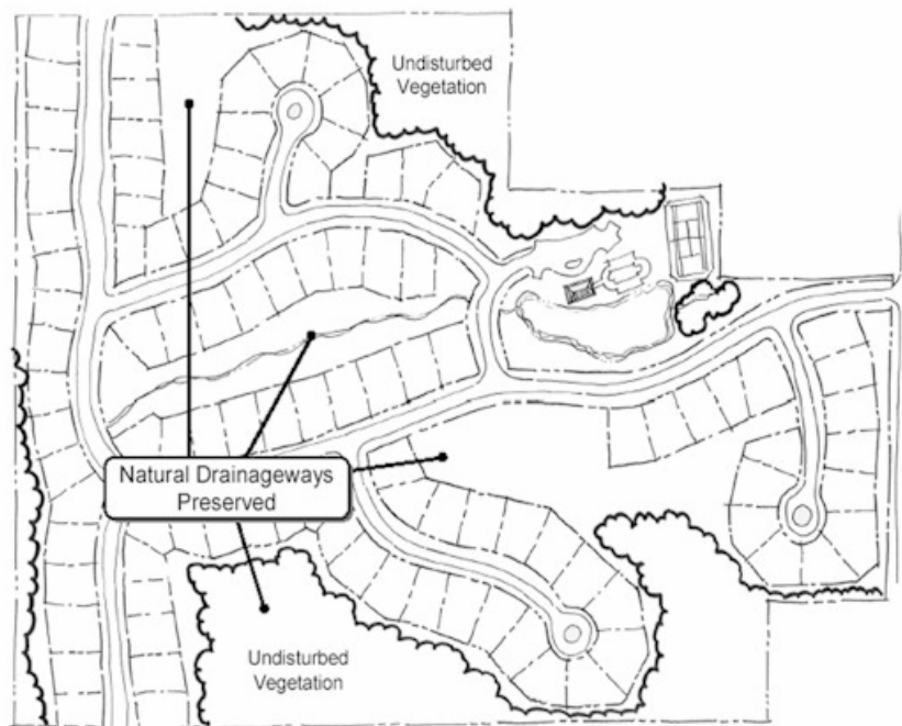
Figure 5.3-1 Protect natural drainage features
