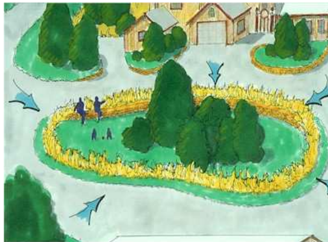
Figure 5.3-6 Natural surface depressions can temporarily store stormwater.
