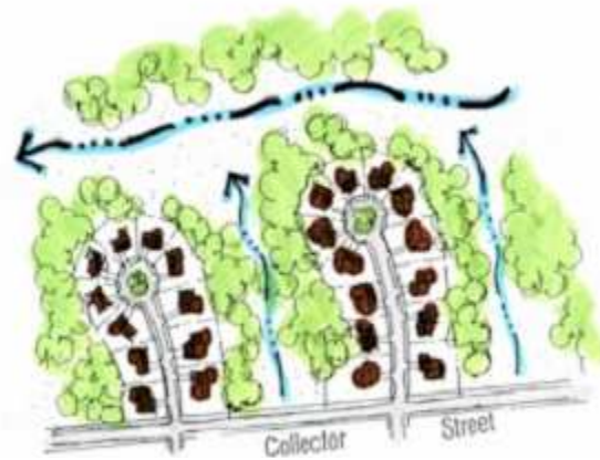
Figure 5.3-5 Natural drainage features can guide the design
